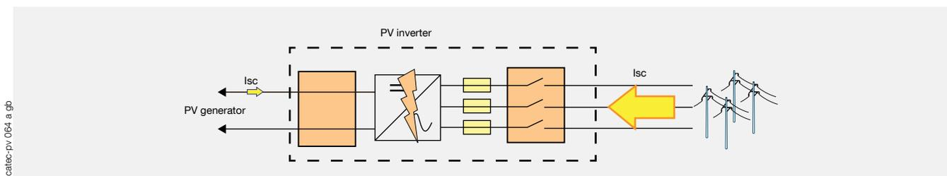
On the AC side, the short-circuit current can be ten times greater than the rated current.
