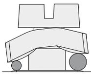
The clamping screw plates of the LED units are provided with a particular "roofing tile" structure and are loosely coupled to the clamping screw. This way, during the wires fixing, the clamping screw plate is able to suit to cables of different diameters and tends to tighten the wires toward the screw instead of permitting them to escape towards the outside.
