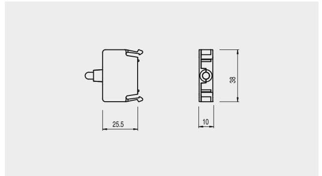
**LED unit for panel mounting, solder connection**
