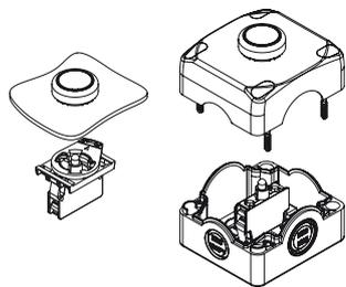
The LED units of the signalling and control devices feature two types of coupling: panel mounting and base mounting.
