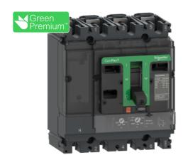
Circuit breaker, ComPacT NSX250F, 36kA/415VAC, 4 poles 4D (neutral fully protected), TMD trip unit 250A
