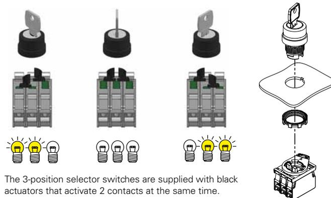
The 3-position selector switches are supplied with black actuators that activate 2 contacts at the same time.
