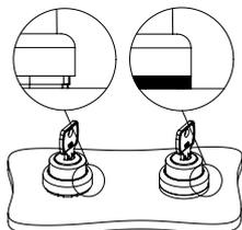
The shaped ring can be used when no label holder or other devices are applied; it prevents dirt and other residues from settling between the selector switch and the panel or housing. This turns out to be particularly useful in the sectors where high standards of cleanness and hygiene are required.
