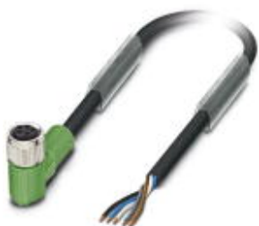
Sensor/actuator cable, 5-position, PUR, black-gray RAL 7021, free cable end, on Socket angled M8, B-coded, cable length: 1.5 m
