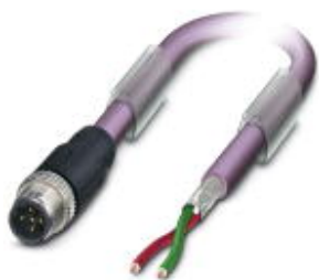
Bus system cable, PROFIBUS, 2-position, PUR halogen-free, violet RAL 4001, shielded, Plug straight M12, B-coded, on free cable end, cable length: 0.8 m
